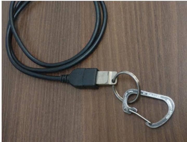
If the laptop snatched the USB magnetic breakaway adapter gets detached from the Laptop that would trigger a udev remove action.
